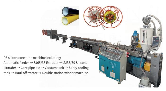
HDPE communication bundle pipe extrusion line including:
